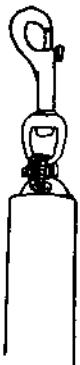
Several different approaches to securing back-up lights to brass or stainless-steel clips using plastic ties
