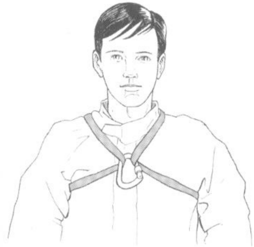
Fig. 337 – Making an emergency chest harness.
